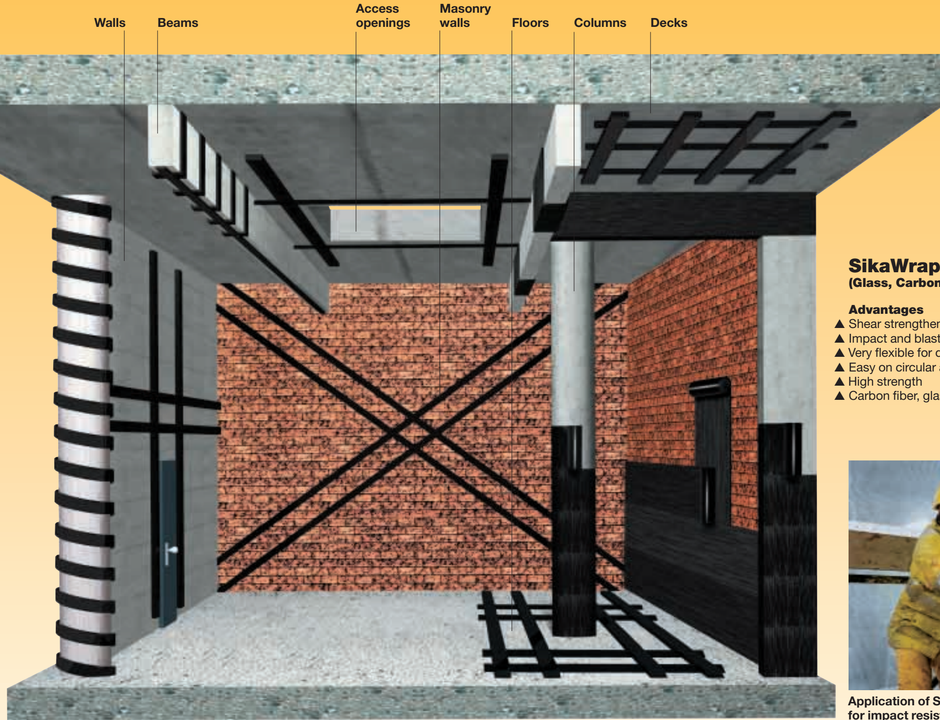
Strengthening of the reinforced concrete slab with the Sika® CarboDur® Plate System (Sikadur-30 adhesive and Sika® CarboDur® plates)
